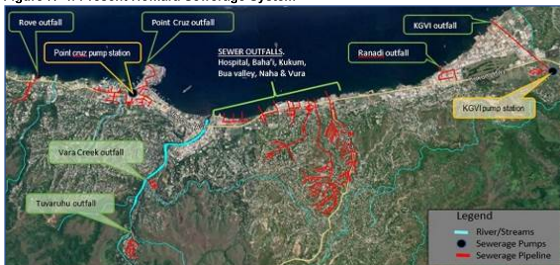
Figure IV-4: Present Honiara Sewerage System
