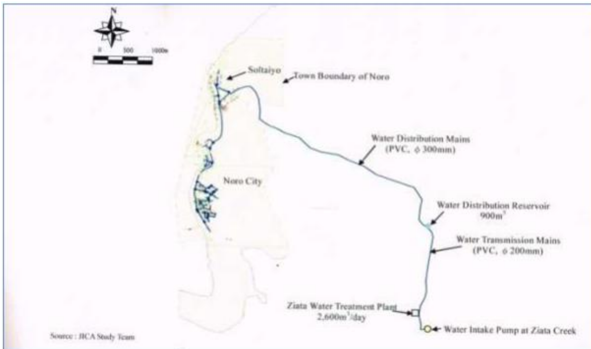
Figure 6-9 Noro Water Supply Schematic
